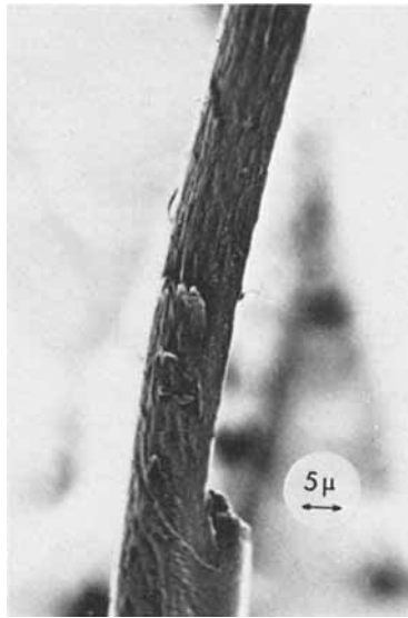
Fig. 14. Initiation points of fatigue fracture on the surface of a Nomex fiber.
